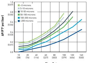
Flow Rate GPM, 1 cps @77°F (Lpm, 1 cps @ 25°C)
