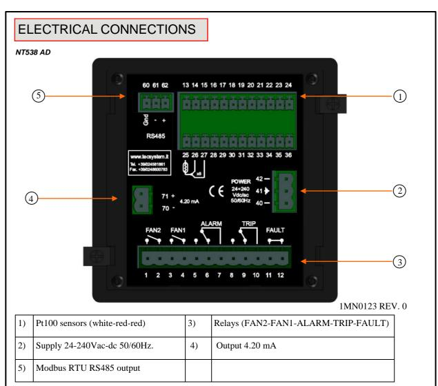
Note: relay contact image in non-alarm condition, with the exception of the FAULT relay that opens: contacts 11-12 open (NO) contacts 11-12 closed (NC) fault condition identification. Read the Alarms and Ventilation paragraph on page 13 and see the opening of the fault contact.
