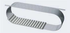
BRECOFLEX BFX versions are manufactured as truly endless timing belts resulting in timing belts with no interruptions or joints. Two bifilar tension members are helically wound throughout the timing belt for superior strength and true tracking. All tension members carry full load throughout the entire timing belt length.
