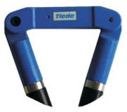
The **MAG-1 magnet** is ideal for the effective magnetization of components for crack detection, particularly where the use of electromagnetic yokes is impractical or prohibited for safety reasons. The hinged arms and rotating angled pole pieces facilitate the local inspection of a diverse range of components such as critical welds and automotive components.
