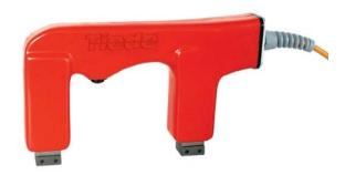
The AC hand yoke **TWM 42 A/N** operates at 42 V supplied from a separate transformer which is connected to a 230 V AC supply. This satisfies the VDE safety regulations so that the TWM 42 A/N can be used for testing invessels, tubes and closed containers.
