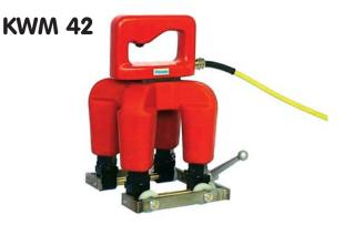
The **cross yoke KWM 42** consists of two AC yokes dis-placed by 90° so that both longitudinal and transverse cracks can be detected in one single operation. Two castors on each magnetic pole maintain a constant air gap and enable the yoke to be moved easily over the test surface. The KWM 42 is powered by a 3-phase supply through a separate transformer.
