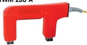
The **TWM 230 A** hand yoke is of similar construction to the TWM-N type, however, the switch on this model can be exchanged when it becomes worn, or faulty. We have also introduced a special switching circuit so that the yoke is switched on when the AC current is passing through zero, thereby greatly extending the life of the switch and the yoke.
