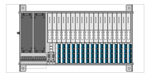
The module rack MT16-2G consists of a backplane and the actual rack system. It can accommodate 2 gateways, 2 power supply units as well as 16 I/O modules. Up to 128 binary inputs/outputs or 64 analog inputs/outputs resp. a mix of both can be connected to it.
