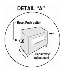
If the instrument trips on start-up, allow the machine to stop. Turn the sensitivity adjustment ¼ turn clockwise, (adjustment for VS94 and VS2EXRB models is located within the box, see **DETAIL B**).
