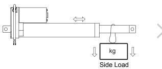
Side load is NOT good for the actuator. In case the actuator rod is exposed to side load the service life time will be reduced.
