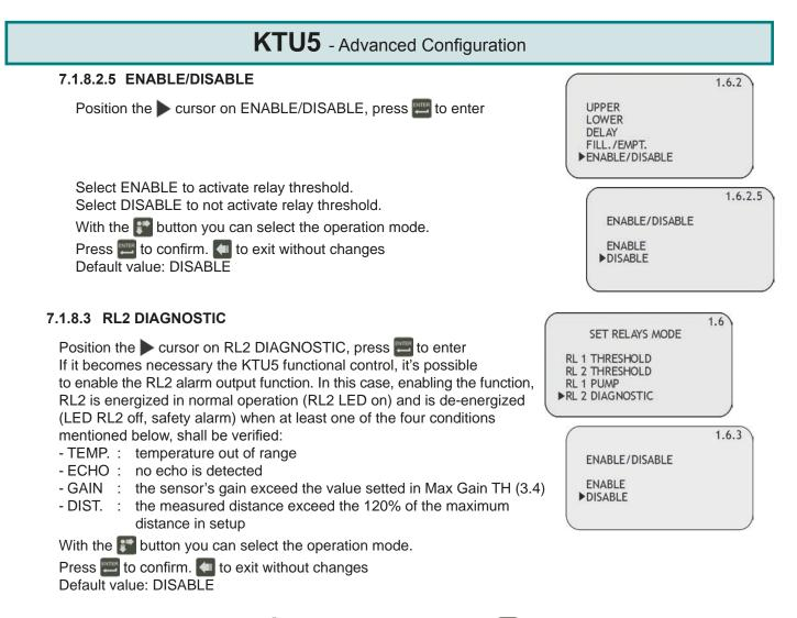
NOTE: when an error occurs, a "!" is flashing on the display: press I to show a message that indicate what kind of error is present. The KTU5 automatically returns to RUN mode.
