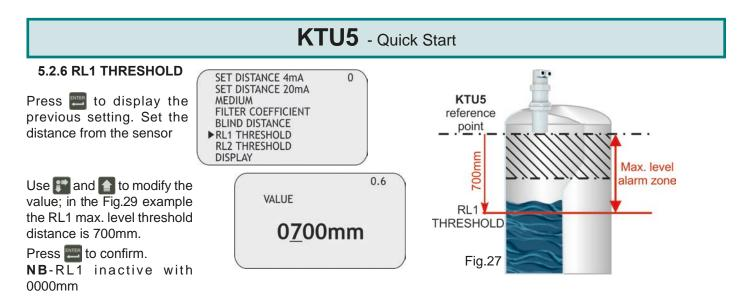
When confirming with the with the maximum level threshold value storage, in the example 700m (figures 29 and 30), the **KTU5** activates RL1 with the following default settings for level alarm threshold:
