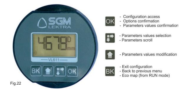
With the VL611 module is possible to access two configuration modes for the KTU5 setting:
