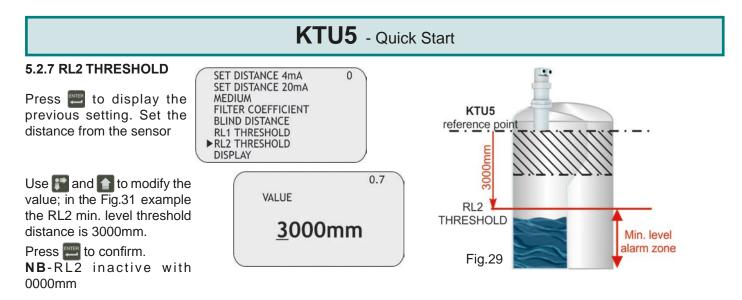
When confirming with the with the maximum level threshold value storage, in the example 3000mm (figures 31 and 32), the **KTU5** activates RL2 with the following default settings for level alarm threshold:
