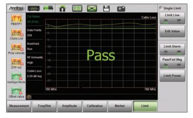
Cable Loss measurement screen (Advanced Mode)
