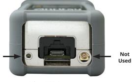
Micro USB Connector With Latch
