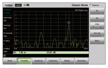
Distance-to-Fault (DTF) measurement screen.
