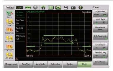
Upper/lower limits and segmented limit lines screen (Advanced Mode Only)
