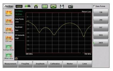
With 1033 datapoints you can extend the maximum Distance-to-Fault range easily
